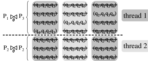
Figure 18: Allocating search spaces using round-robin inner for building P_4 to two threads.
