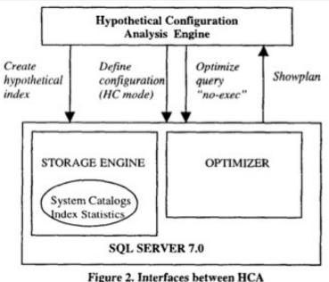
Figure 2. Interfaces between HCA Engine and SQL Server
